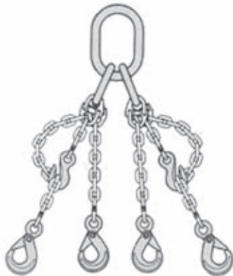
Four Legged Sling with Eye Self-locking Hooks. Available with or without BEG Eye Grab Hooks.
